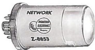
SPECIAL PLUG-IN CIRCUITS CAN BE HOUSED IN STANDARD CONTAINERS
